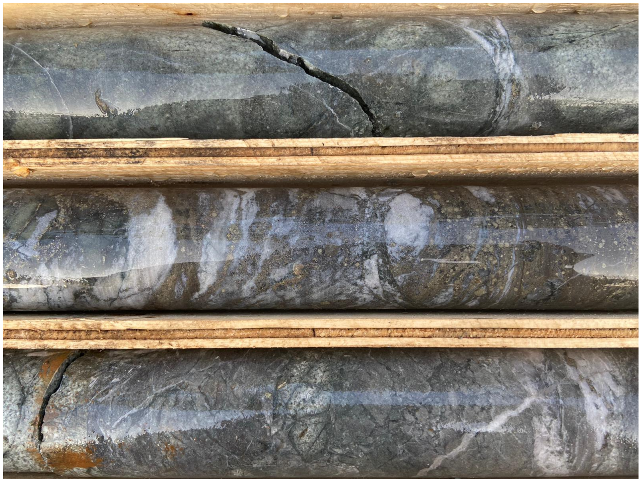
Figure 4: GH-DDH-21-004: 353.9m to 357.4m. Massive pyrite overprinting refractured early quartz veins with a secondary pyrite mineralizing event with brighter coloured blebby pyrite.
