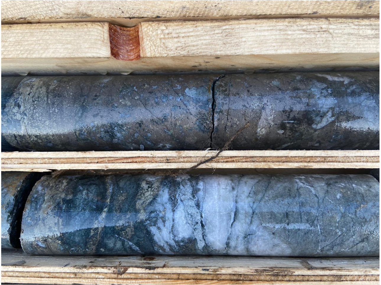
Figure 5: GH-DDH-21-004: 353.9m to 357.4m. (Top row) Massive dark brass coloured pyrrhotite with semi-massive pyrite along margins overprinting an earlier tourmaline-silica breccia. (Bottom Row) strong vein marginal pyrite lesser pyrrhotite mineralization.
