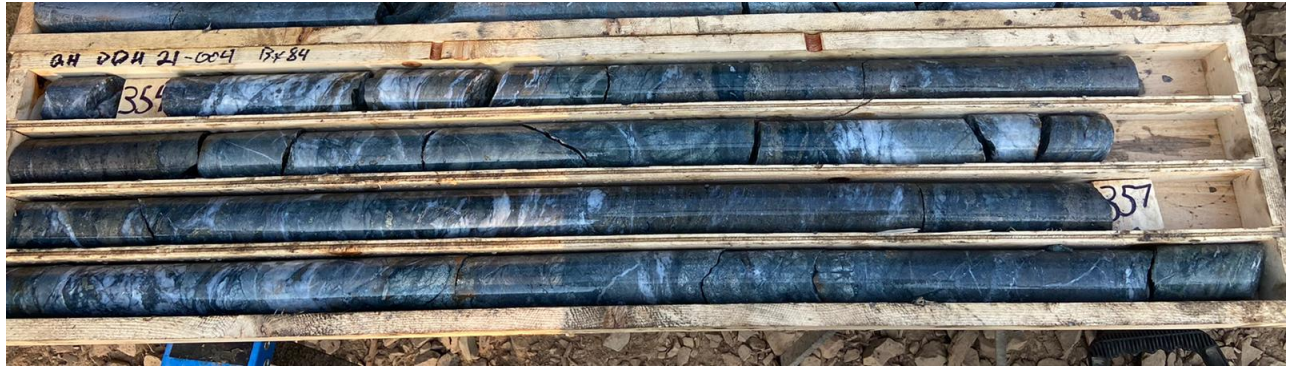
Figure 4: GH-DDH-21-004: 353.9m to 357.4m. Massive pyrite overprinting refractured early quartz veins with a secondary pyrite mineralizing event with brighter coloured blebby pyrite.
