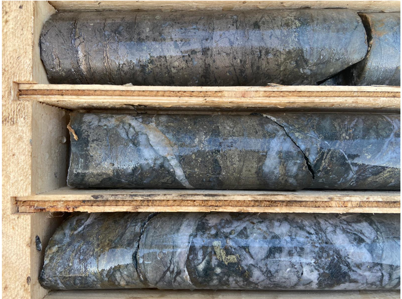
Figure 6: GH-DDH-21-004: 353.9m to 357.4m. (Top row) Massive dark brass coloured pyrrhotite with semi-massive pyrite along margins overprinting an earlier tourmaline-silica breccia. (Middle Row) strong vein marginal massive pyrite lesser pyrrhotite mineralization. Bottom Row: Pyrite lesser chalcopyrite mineralized overprint of earlier tourmaline-grey silica hydrothermal breccia.
